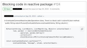
Figure 4: Blocking call due to a block() operator [7].
